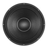
This next evolution subwoofer uses a new, longer, four layer aluminum voice coil. The result is less heat, more energy in the gap, higher sensitivity, higher power handling, lower distortion and better overall performance. The 18DS100 features a 36.5 mm long, 4 inch diameter (100mm) Copper Clad Aluminum Wire voice coil. With a 1500watt AES power rating, 97.5 dB sensitivity, and over 14.0mm of Xvar, this high energy subwoofer is a significant step forward from similar models in the B&C range.
